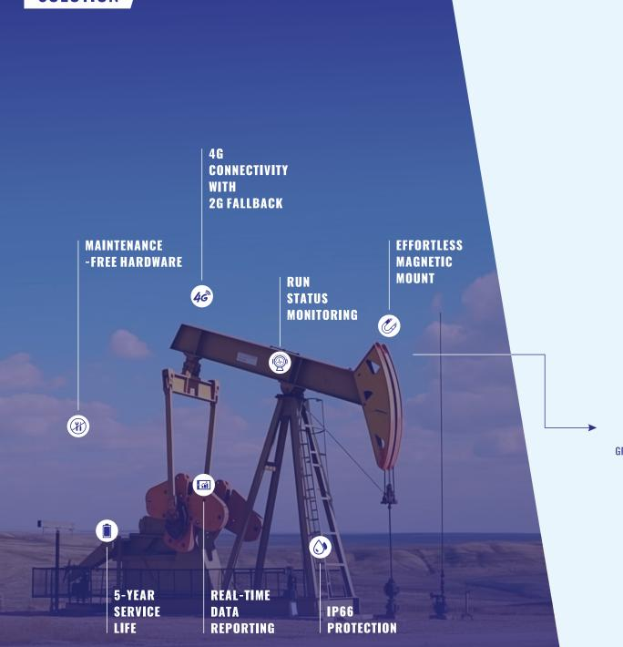
**DEVICE** Run time efficiency monitoring devices installed on the walking beams collect the run status data (start, stop, swing) of the pumpjacks in real-time and upload the data using the cellular network to the cloud server.
