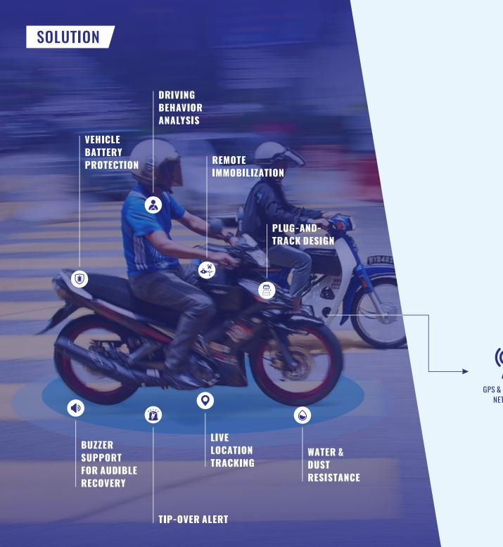
**DEVICE** Jimi IoT's telematics devices installed on electric scooters, bikes, mopeds, and other two-wheelers interact with and collect data such as locations, battery status and faults and upload these data to a cloud-based platform.
